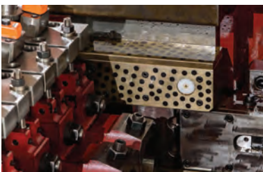
◆ Main Slide Shim-Plated with Self-Lubricant Graphite
